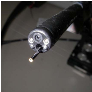
Figure 01: Tip of Conventional Endoscope, usually the diameter is 4 mm to 6 mm
